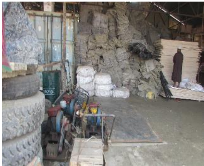
Figure 1 Storage with flammable items and fuel together
