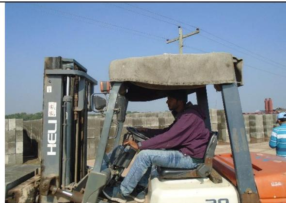
Forklift moves in the work site at Tafalbari CC block manufacturing yard under polder-35/1. But no signal man presence in the worksite and vehicle driver did not use any PPE.
