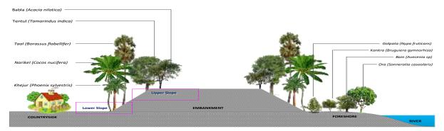
Figure 10.2: Typical cross section of Embankment slope and Foreshore Afforestation
