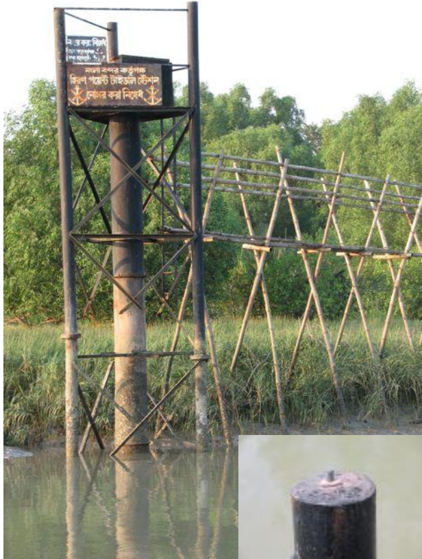
Figure 2-7: Tide gauge at Hiron Point. Monument pin (inset was installed on far cement-filled support column).
