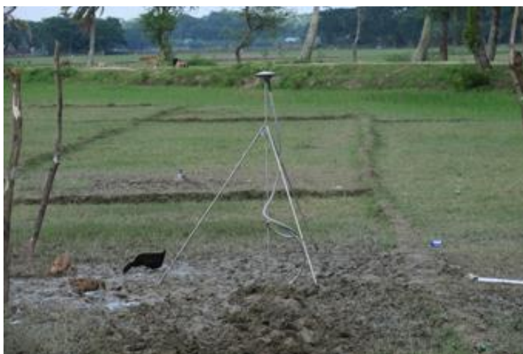
Figure 2-6: GPS mounted on rod identical to that of RSET, visible in next field. A tripod was added for stability, but bracing has a cylinder that allows free motion of the rod to measure deep subsidence.
