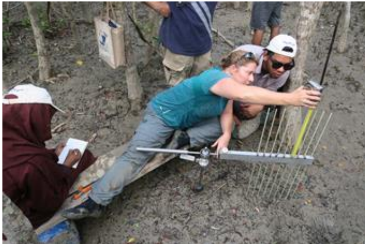
Figure 2-8: Carol Wilson measuring the height of one of the fingers on an RSET arm at Katka. Carol and Sharmin are on board to avoid touching the measurement area around the RSET.
