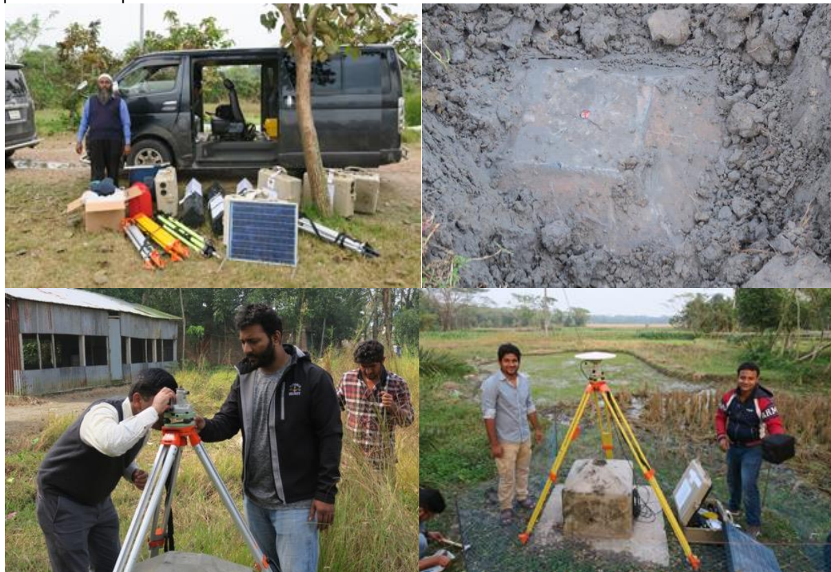
Figure 2-11: A). The suite of surveying equipment laid out in front of one of our vans and driver. B) Close up of the buried monument at site 202. The brass pin with an X marking the measurement point is visible in the center of the concrete monument. C) Mondal and Sober using the tribrach and optical plummet on the tripod to center and level the antenna monument. D) Masud and Hasnat next to a completed station. The still open box holds the GPS receiver and power supply equipment. The solar panel is next to it. and everything is surrounded by a fence to keep the site from being disturbed.
