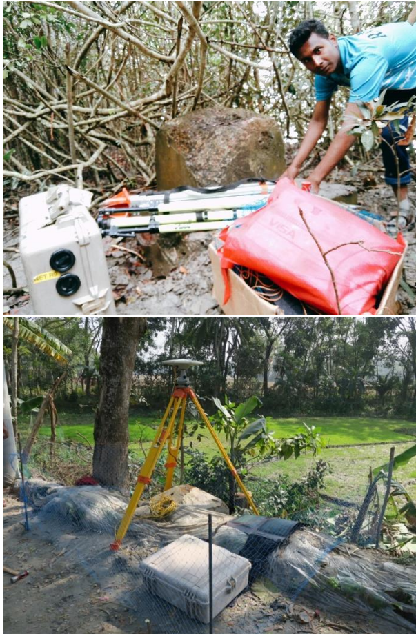
Photograph -1 A) Badly eroded monument GPS 140 in the Subdarbans. B) Monument GPS 194 along the edge of a road. There is concern about whether some monuments, such as this one may be disturbed by local ground motions.
