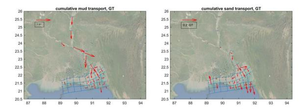
Figure 4.2 Yearly cumulative mud transports (left pane) and sand transports (right pane) in macro scale model, mind the different vector scales
