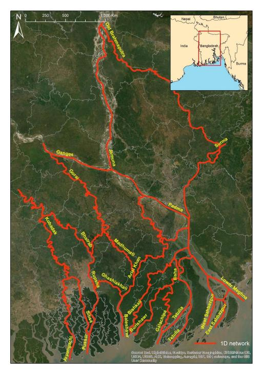
Figure 4.4 River network for the Delft3D-FM 1D model.
