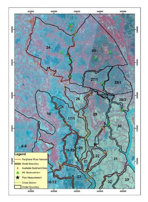
Figure 4.19 River Network for Mike 11 Model Extracted from SWRM
