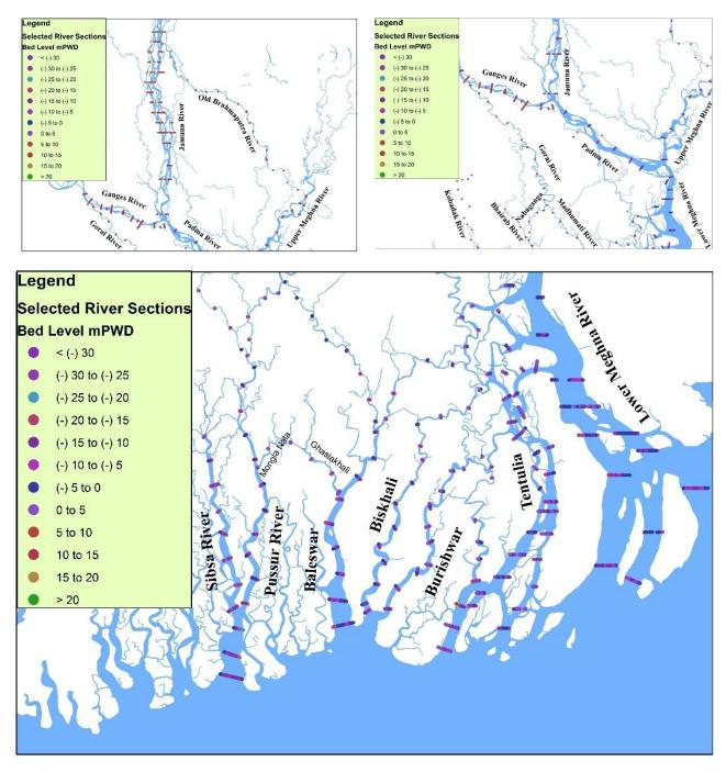
Figure 4.5 Maps showing the selected measured cross sections imposed on the model.
