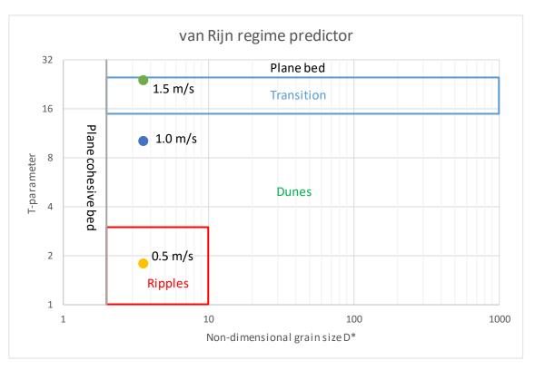
Figure 4.14 Application of the van Rijn regime predictor for the point bars in Pussur River.
