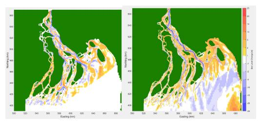
Figure 4.9 Observed (left panel) and simulated (right panel) bed level changes, 2000-2009, settings 2
