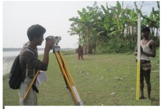
Figure: Embankment Cross section Survey
