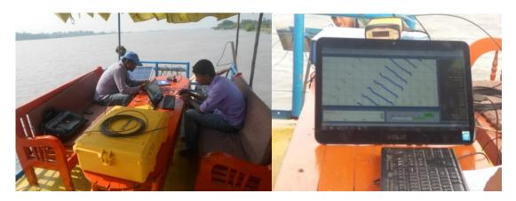
Figure: Bathymetry Survey at the surrounding river of Polder 29.
