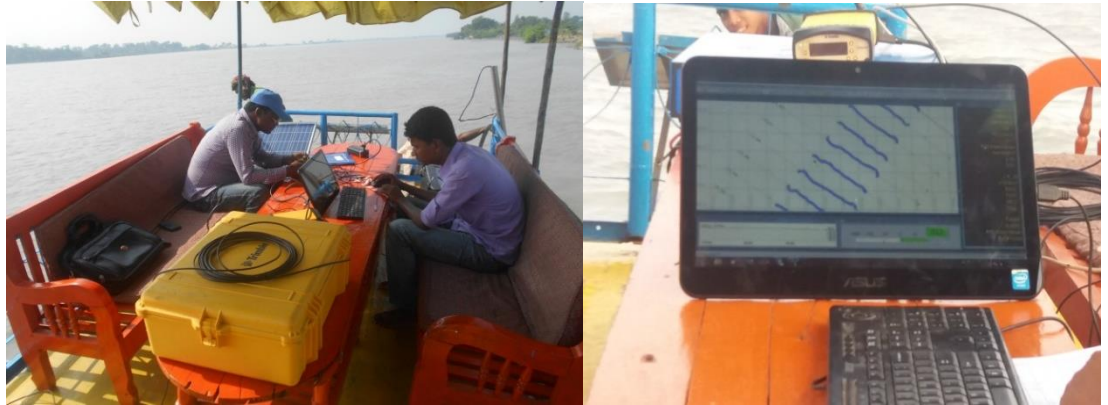
Figure: Bathymetry Survey at the surrounding river of Polder 29.
