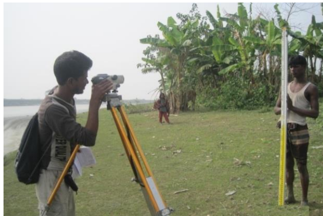
Figure: Embankment Cross section Survey
