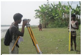
Figure: Embankment Cross section Survey
