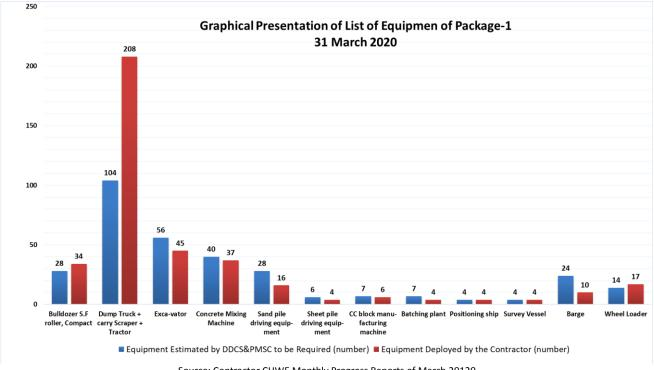
Figure 4: Comparison of Equipment Available and Required - Package 01
