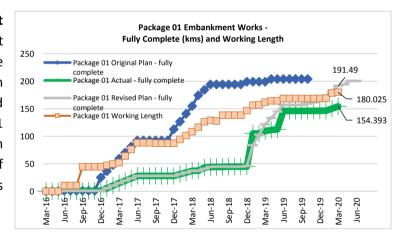
While Package 01 has achieved 80.9% progress for **embankment earthworks** in cubic meter terms, there is variability across polders. Polder 35/3 is the furthest advanced at 94.0% complete, Polder 33 at 83.85% complete, then Polder 32 at 77.55% and 35/1 approaching 74.80%.
