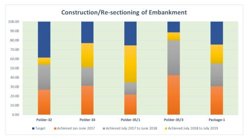
Figure 3-33: Construction/Re-sectioning of Embankment of Package-1
