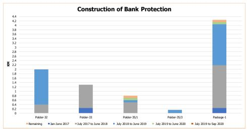
Figure 3-7: Construction of Bank Protection works of Package-1
